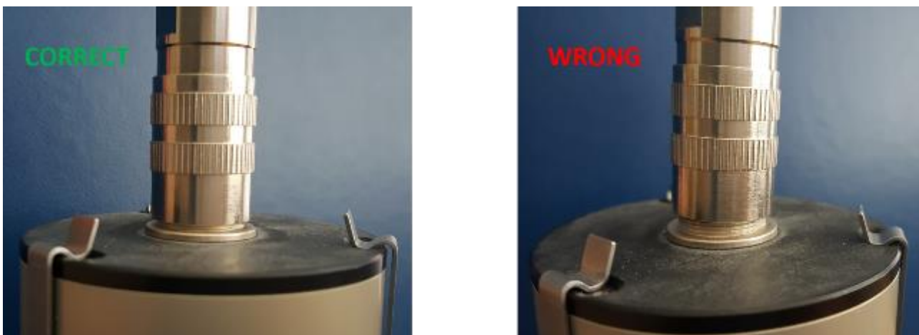
Figure 6: Left: Correctly mounted plug. Right: Plug screw part is tilted and tightened but the plug does not seal at all!
