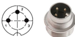
Figure 5: Three pin connector on actuator side. Pin assignment: pin 1 =GND, pin 2 = NC, pin 3 = +24VDC.
